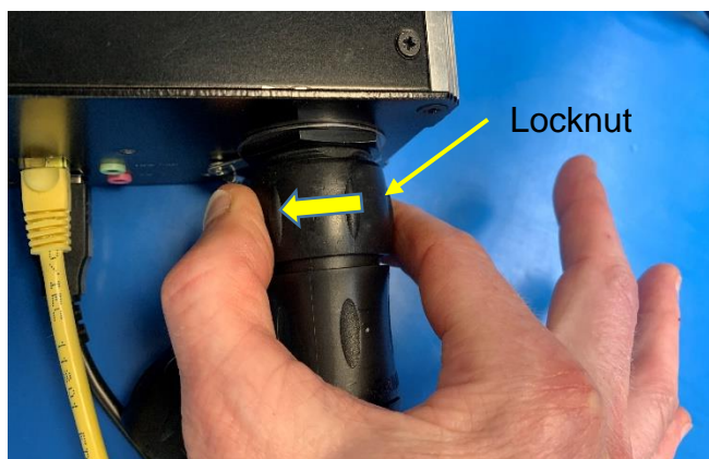
Figure 16: Disconnecting Souriau connectors
