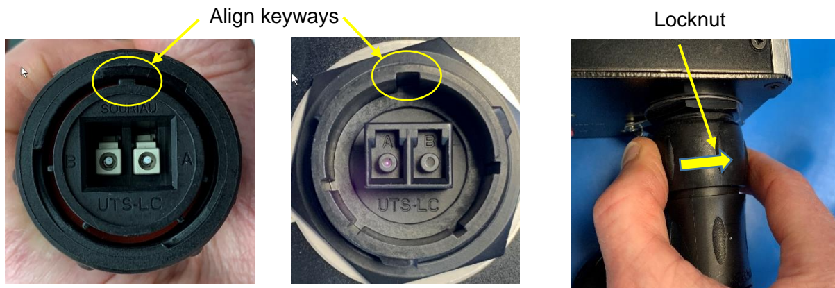
Figure 19: Reconnecting the Souriau connectors
