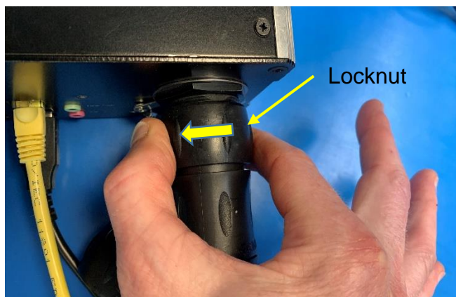
Figure 10: Disconnecting Souriau connectors
