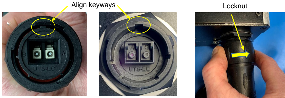
Figure 13: Reconnecting the Souriau connectors
