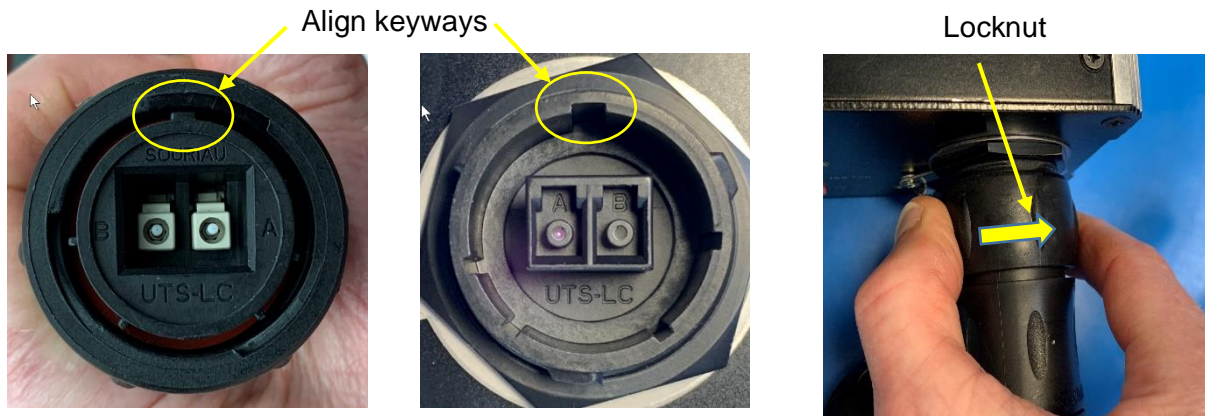
Figure 20: Reconnecting the Souriau connectors
