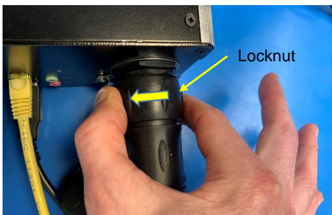
Figure 17: Disconnecting Souriau connectors
